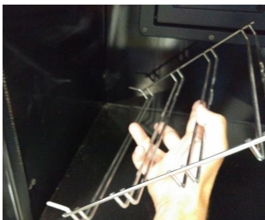
Figure No.21 - Removal of the brackets and self-cleaning sides
